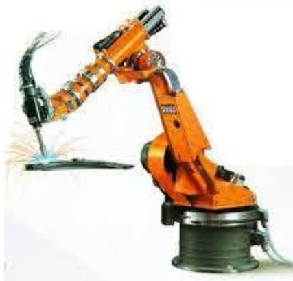
Fig.3. Industrial robot used in welding operations
